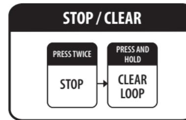
**NOTE :** When the loop is clear, DITTO turns off and returns to true bypass
