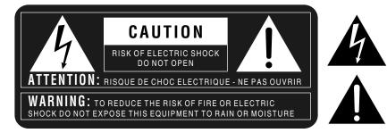
The lightning flash with arrowhead symbol, within an equilateral triangle, is intended to alert the user to the presence of uninsulated idangerous voltageî within the productis enclosure that may be of sufficient magnitude to constitute a risk of electric shock to persons.
